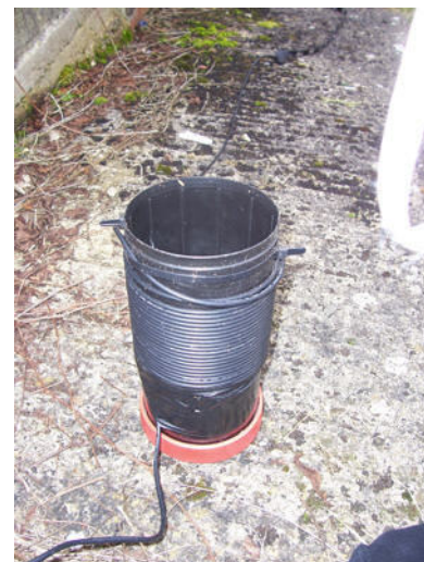
RF Feed line Choke used by G7FEK.
