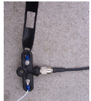
A Typical G7FEK antenna feed point before weatherproofing with self amalgamating tape
