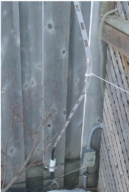
"Taking up the slack" - This is the feedpoint of Scott's (VE3SCP) version of the G7FEK antenna.
